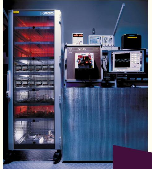
**Saturn**™ is a bespoke set of test equipment designed and developed by AGD Systems. It is dedicated to the testing of the 307 detector range and 100% of these units manufactured at AGD are Certified by Saturn.
